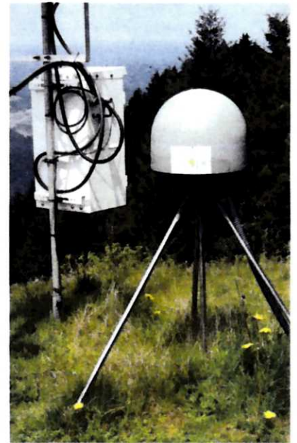
The Geosensor is used to detect seismic activities.
